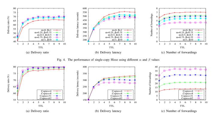
Fig. 5. The performance of multi-copy Hisso using different number of copies
