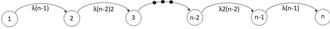
Fig. 3. Markov chain where each state X_i represents i nodes having received MTB
